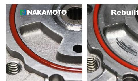
If not remanufactured properly, worn surfaces will continue to generate debris and can cause permanent damage to the steering system.
